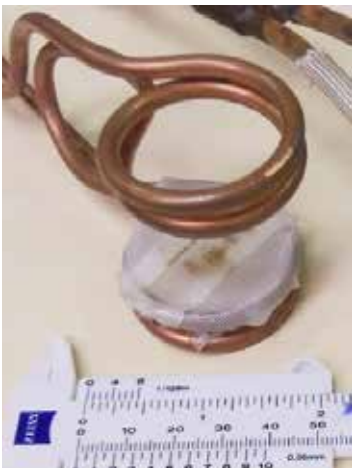
The split helical coil enabled easy loading.
