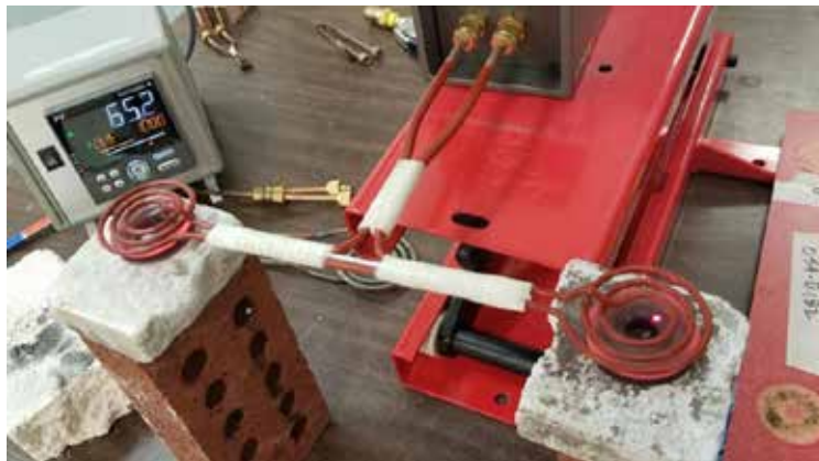
The test setup for this shrink fitting application.
