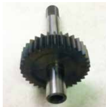
The gear and shaft after shrink fitting.
