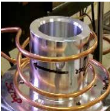
The aluminum hub inside the induction coil.
