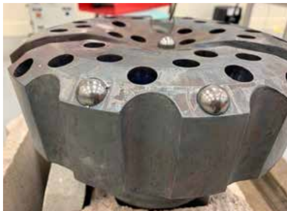
The drill head with carbide bits.
